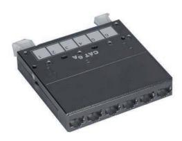
The 6 Port Screened Category 6A Pre-termination ready Cassette offers a flexible and quick way to terminate and install structured cabling. Manufactured from high impact flame retardant plastic, the modules use IDC punch downs for the termination of the copper cables. The Cassettes are easily fitted and removed from the rear of the patch panel by activating re-lease latches.
